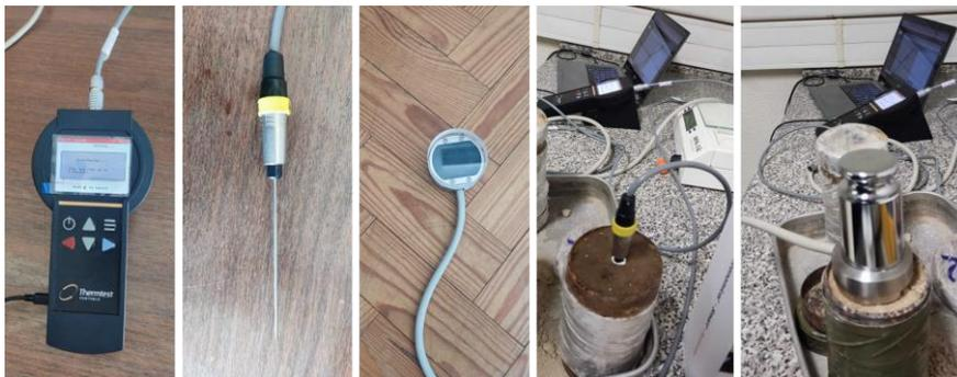
**Figure 2** – Needle and plane source probes with their respective test setups.
