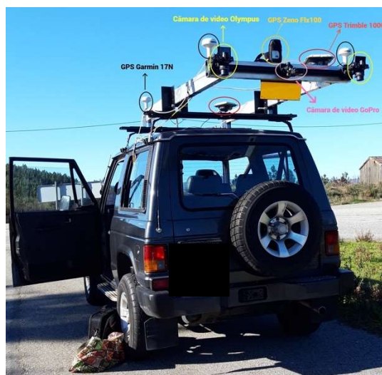
Figure 1 – Instrumented ground vehicle and the arrangement of equipment used in the survey.
