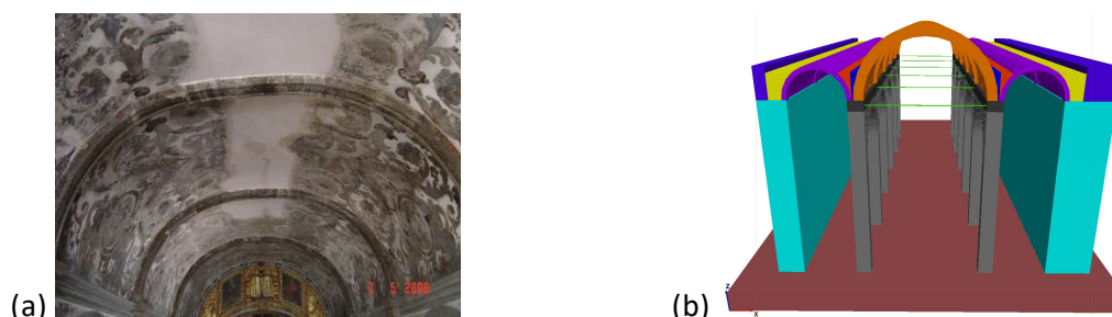
Figure 2 – (a) Church of Bucelas; (b) Reinforcement solution.
